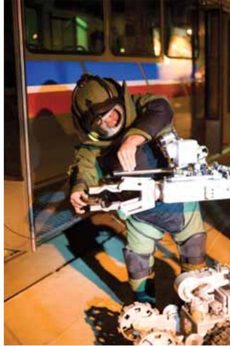
An explosives ordnance technician readies an explosives detection and removal robot during a video production for the Transportation Security Administration by the FLTEC's Media Support Division.
