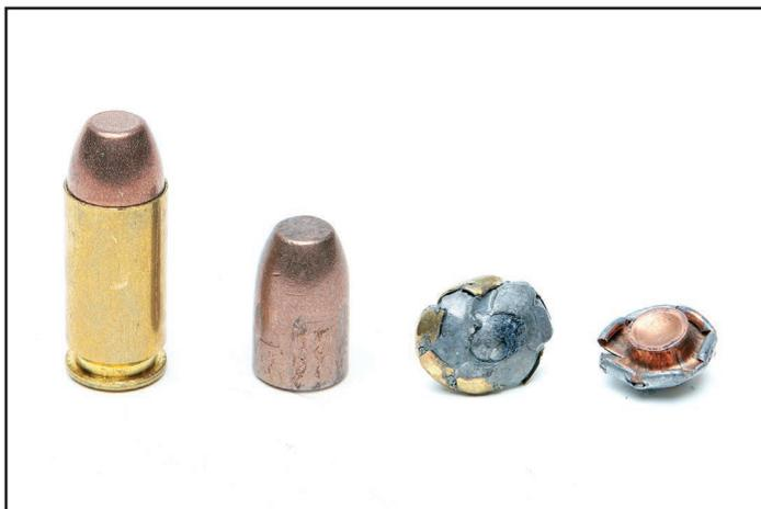
*Sample of .40 cal lead ammunition in its shell casing, removed and after impact.*
