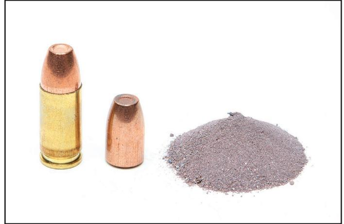
*Sample of 9mm frangible ammunition in its shell casing, removed and after impact.*
