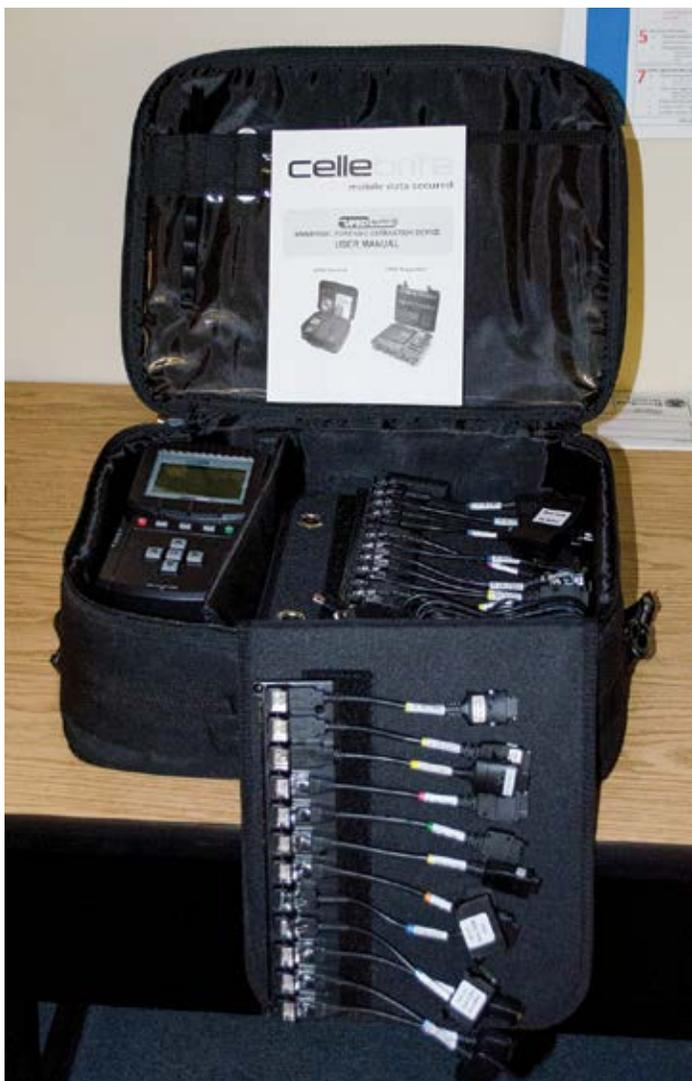
A Cellebrite UFED kit shown with many of the different cables used to connect the device to as many as 6,500 different cellular phones in use today.
