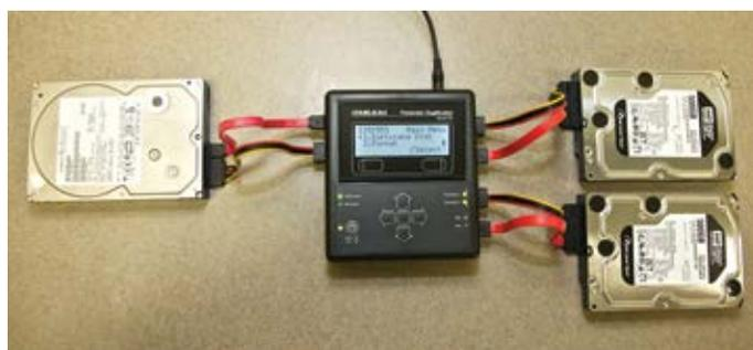
The TD2 handheld hard disk imager shown preparing a forensic copy of the suspect hard disk on the left and sending two copies to the connected hard disks on the right.
