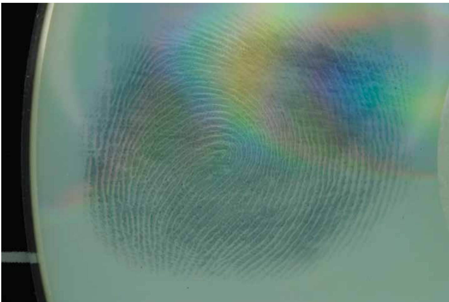
ABOVE: An example of diffused lighting sources to document latent fingerprints on a reflective surface. OPPOSITE: An example of using laser light to track ballistic trajectories for crime scene analysis and reconstruction.
