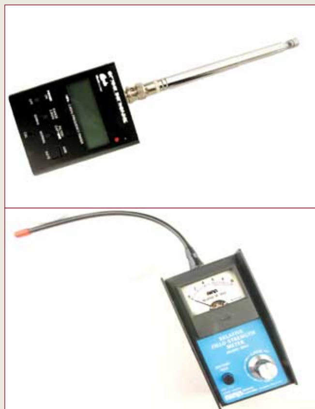
TOP: A frequency detector is an electronic "bug detector" that will act as frequency sweepers. If any operating RF transmitting devices are detected the device will tell you in which frequency the bug is operating. ABOVE: A field strength meter is an easy-to-use meter. It shows the strength of the actual field being radiated from an active RF antenna. You can use it to determine the basic radiation pattern of your antenna and see which direction your signal is strongest. You can make changes to your antenna and instantly know if it radiates better.
