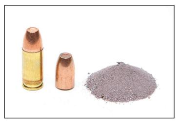
Sample of 9mm frangible ammunition in its shell casing, removed and after impact.
