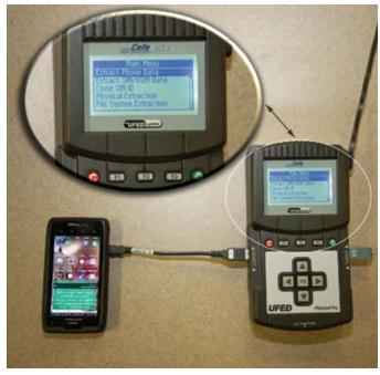
A Cellebrite UFED connected to a Smartphone on the left; preparing to copy data from the phone to a connected USB thumb drive on the right.
