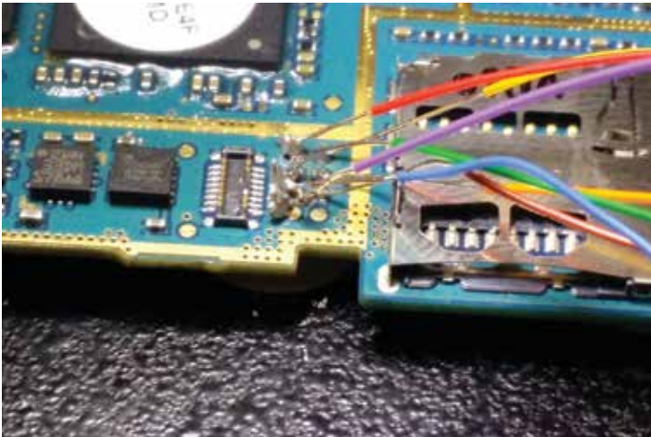
Above photo: Example of student's first soldering attempt using JTAG. Right photo: How to identify relevant memory chips for chipoff analysis.
