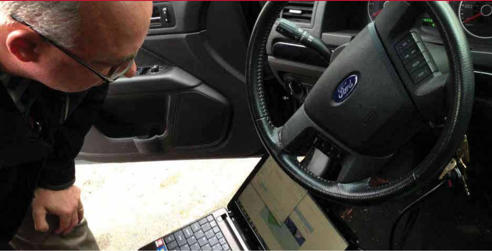
Laptop is connected to vehicle infotainment system to obtain digital evidence.
