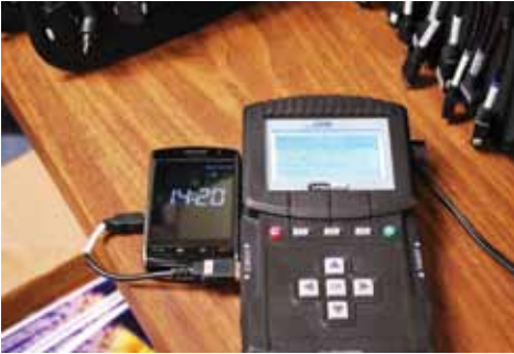
Top Photo: The Susteem cell phone forensic analysis tool connected to a BlackBerry cellular device, pending analysis. This is one of the tools issued to students in FLETC's Mobile Device Investigations Program.
